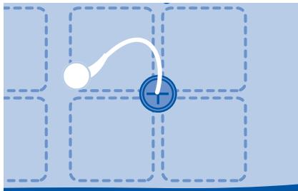
**3 Clip the electrodes to the snaps of the accessory**
